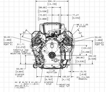
ENGINE MOUNTING SURFACE (PTO END)
